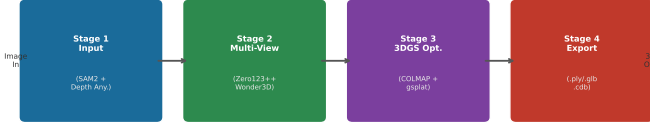
Fig. 1. Orb four-stage pipeline: Input \rightarrow Multi-View \rightarrow 3DGS Optimization \rightarrow Export.
